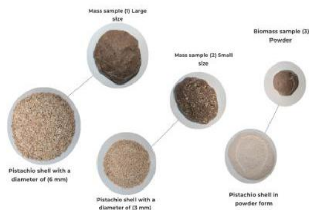
Figure 2. Particle size reduction sequence of pistachio shells and their subsequent agglomeration into biomass.
