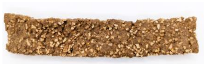
Figure 4. Pistachio shell sheet with fine granulometry (3 mm).
