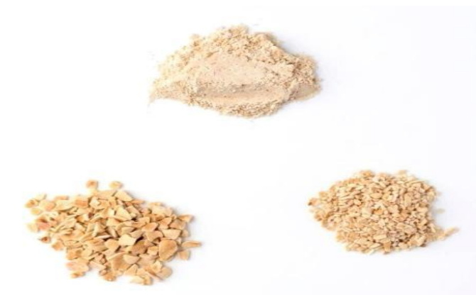
Figure 1. Variation of particle size and granulometry of pistachio shells.
